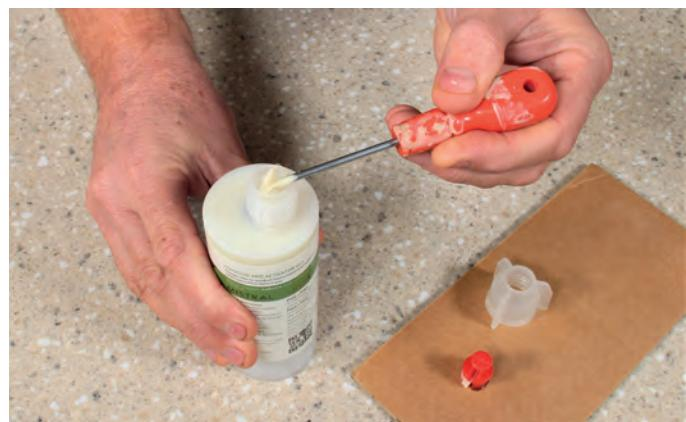
Attach the nozzle to the end of the adhesive cartridge.
