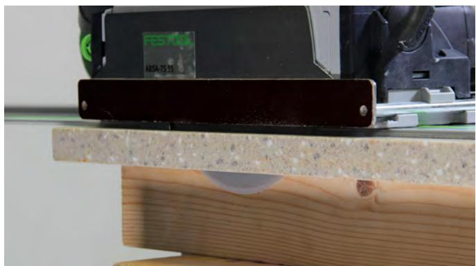
If using a slow or soft start circular saw, make sure you obtain full speed before starting. Perform the cut at a slow and even pace until the back of the blade has fully passed through the worktop.
