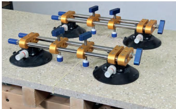
If you are jointing longer pieces you will need additional sets of seaming tools or sash clamps to ensure that the joint is sufficiently pulled together all the way along.
