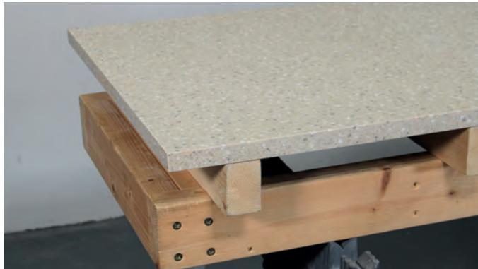
Clamp the worktop and support blocks to the bench and then clamp the straight edge to the worktop. Ensure there is no movement during the machining process.
