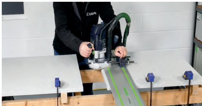
We recommend the use of our spiral router cutters, as they are designed to apply the router's power more evenly, to create a smoother result, and their up-cut action aids effective extraction.
