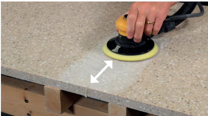
**Never tilt the sander and use just the outside edge for quick removal. This can cause dips in the surface which are extremely difficult to remove.**
