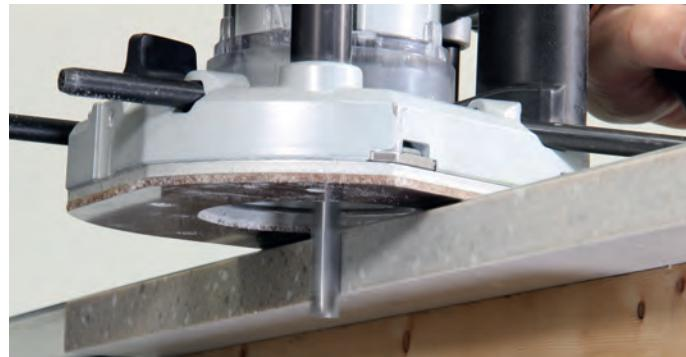
Starting at the front edge of the worktop, perform the trimming operation keeping the router running along the straight edge/guide rail throughout.
