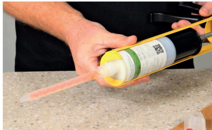
Place the threaded cap back over the self-mixing nozzle and lock the nozzle into place.
